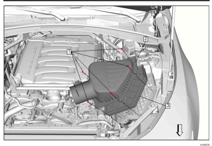
**Note:** The MAF sensor must stay connected so that no DTCs will set.
