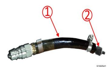
8. Install the DT-45096-31 adapter (1) to the DT-51190 fluid fill adapter (2).
