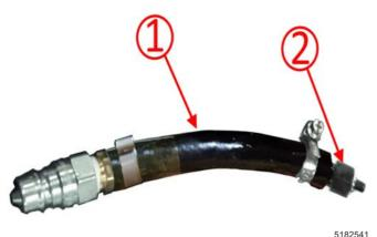
9. Install the DT-45096-31 adapter (1) to the DT-51190 fluid fill adapter (2).
